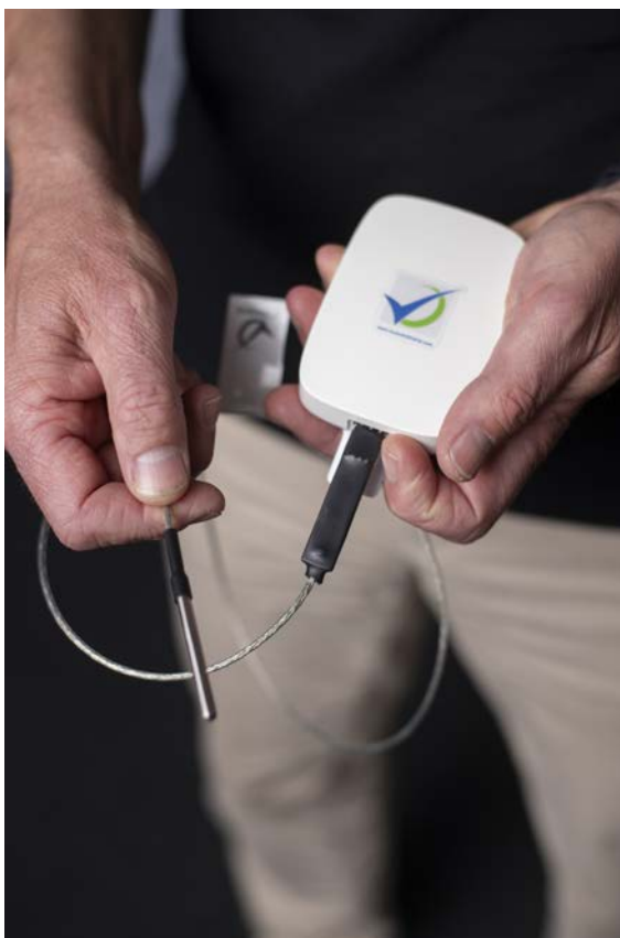
Pt100 sensors in these cryogenic liquid-nitrogen tanks – as used at IVF clinics and shown here – keep the temperature at -196^{\circ}\text{C} . If it rises, the ICU “Boomerang” system sounds an alarm to prompt nitrogen refill.
