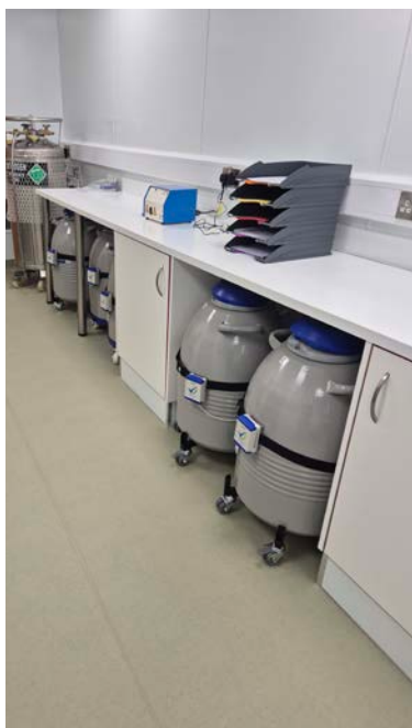
Pt100 sensors in these cryogenic liquid-nitrogen tanks – as used at IVF clinics and shown here – keep the temperature at -196^{\circ}\text{C} . If it rises, the ICU “Boomerang” system sounds an alarm to prompt nitrogen refill.
