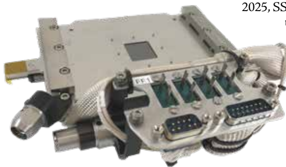
A very compact gradient furnace that SSC built for these experiments includes small heaters where thermocouples from Pentronic are installed. The thermocouples must not be larger than 0.5 millimeters in diameter.
