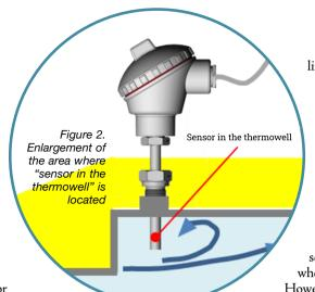
limits the convective heat flow to the thermowell and thermocouple. This means that the sensor reacts slowly and its response time can be fairly long. In the case of dirty fluids, the dirt often accumulates in the wake area. However, one advantage of this particular installation is that it leads to a minimal extra pressure drop.
