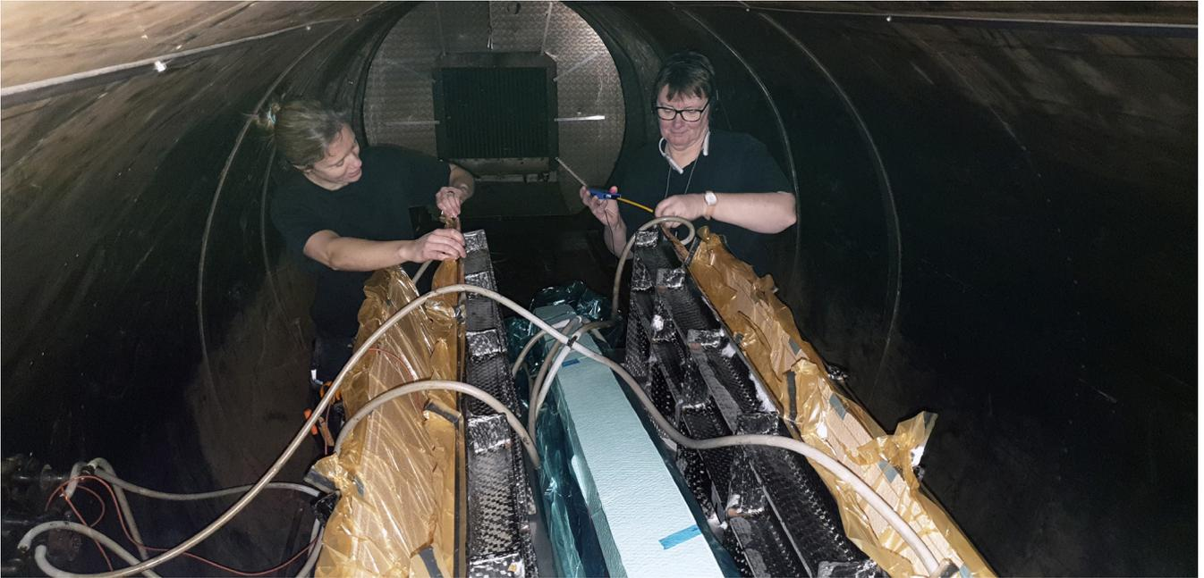
*Mounting temperature sensors inside the 35-metre-long autoclave for making boat masts.*
