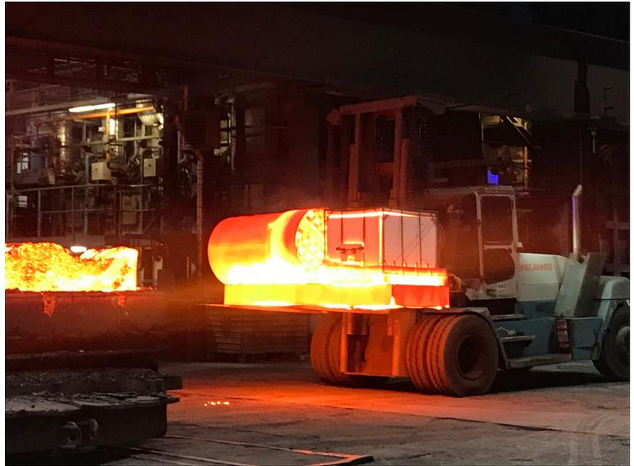
Here the heat-treated steel together with its accompanying measurement equipment is being retrieved from the furnace by a forklift truck. The load of about seven tonnes is still at a temperature of over 1000 °C.
