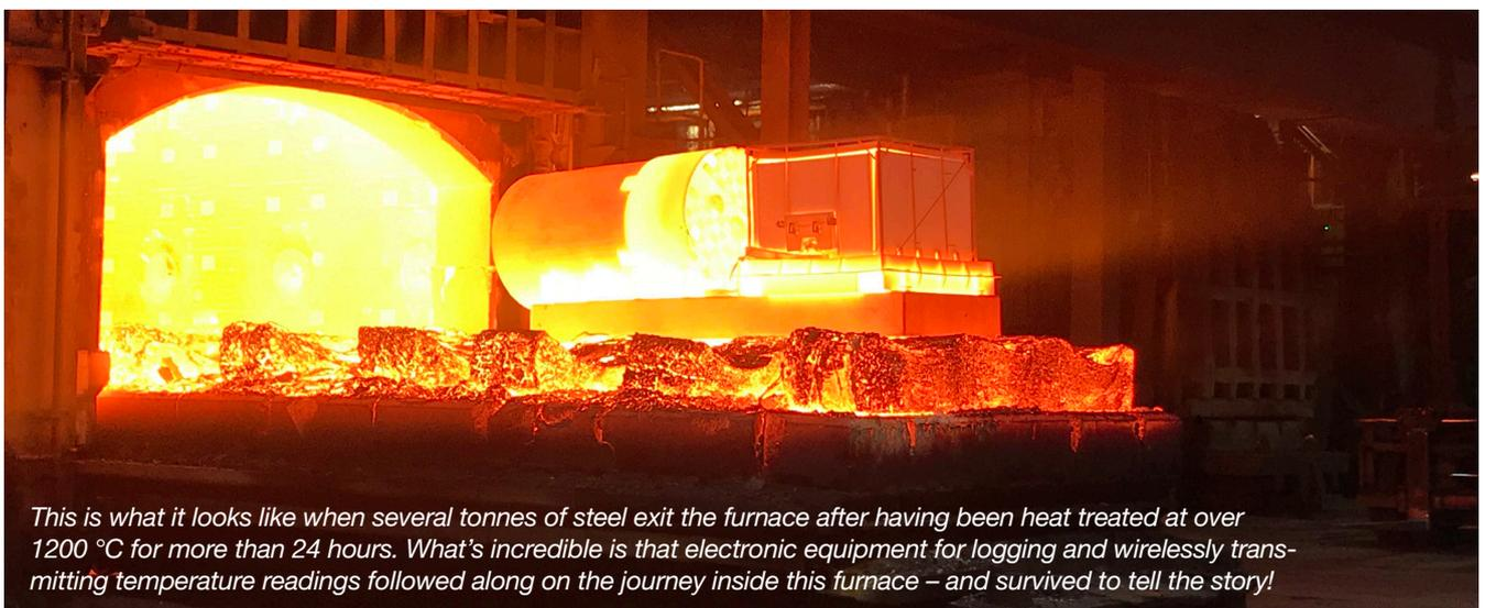
*This is what it looks like when several tonnes of steel exit the furnace after having been heat treated at over 1200 °C for more than 24 hours. What's incredible is that electronic equipment for logging and wirelessly transmitting temperature readings followed along on the journey inside this furnace – and survived to tell the story!*
