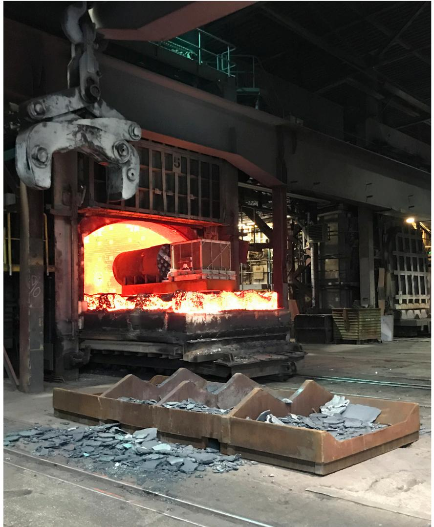
*A steel ingot with measurement equipment heading into the furnace for heat treatment.*
