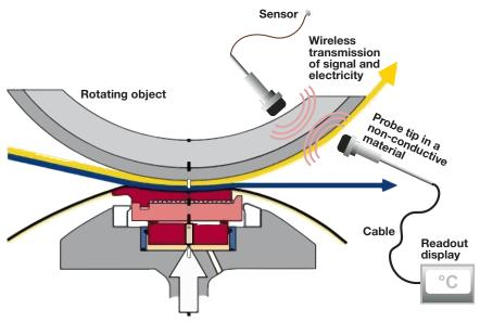
Using digital technology also makes it possible to connect the sensors to a bus system in order to reduce the need for laying cables in multisensor applications. Digital signal transmission eliminates measurement errors in the signal chain by digitally transmitting the sensor signal all the way from the sensor to the measuring or control system. A number of Pentronic's customer have chosen this type of technology for their applications.
