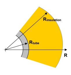
Heat flow as a function of radius, Q(R), for a  $\emptyset$  40 mm tube with wet insulation.
