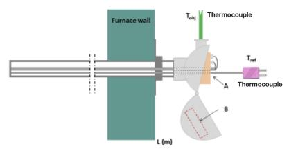
The reference sensor is inserted inside the extra tube that is inside the existing terminal block, see A.
