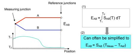
The figure shows at left a thermocouple that is exposed to a temperature gradient. The signal output EAB is generally expressed by an integral, but can often be simplified to the sensitivity (the Seebeck coefficient multiplied by the temperature difference between the measuring and reference junctions).
