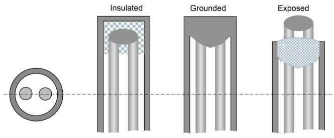
Sheathed thermocouples with the measuring junction's locations shown in cross-section. The diameter of the wires is normally approx. 20% of the sheath's outer diameter. The sheath's thickness is normally approx. 10-15% of the outer diameter.
