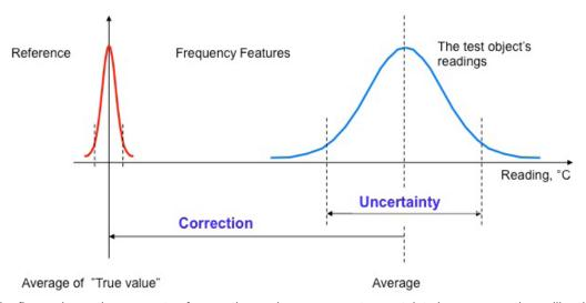
The figure shows the concepts of correction and measurement uncertainty in a comparative calibration. You obtain the spread around the mean values by repeating the readings a large number of times. The spread is caused by the chance measurement errors that are introduced with every reading.
