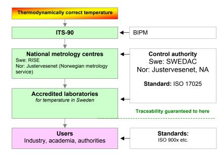
This figure shows how temperature is made traceable to ITS-90 via various calibration bodies. The link to the thermodynamic temperature is via BIPM's research project.
