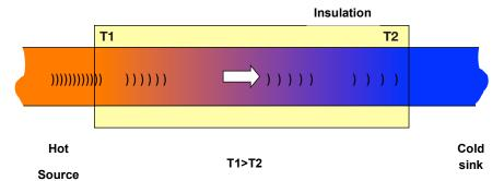
Heat transfer by conduction. Vibrational energy is transferred from atom to atom. In general, metals are the best conductors. Gases are the worst.
