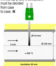
The probe tip has become sooty from the flow of exhaust in the pipe. How does this affect the temperature measurement?
