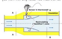
careful when installing thermowells and other components that disrupt the flow. One example is discussed in [Ref 2].
