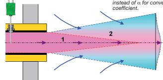
1 = the core jet and 2 = the mixed flow area where the core flow combines with the ambient air outside the outer edge of the jet.
