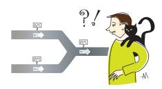
ANSWER: IIn this case we can rule out any fault in the measurement system. If the sensor's attachment to the wall is colder than the incoming air streams, a heat flow along the sensor to the wall could reduce the temperature reading. Radiation from the sensor to the cold walls of the pipe containing the mixed air stream could also cause this effect.
