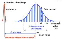
Diagram 1. A theoretical histogram of a calibration in which the columns represent the number of times that the same measured value has occurred. The correction term and measurement uncertainty must be stated in order for the calibration to be complete and meet the requirements of quality standards such as ISO 9000.
