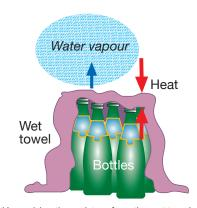
Vapourizing the moisture from the wet towel requires heat, which is taken partly from the bottles.
