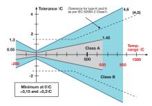
Diagram 2. Tolerances for a Pt100 according to IEC 60751 classes A (grey) and B (blue).
