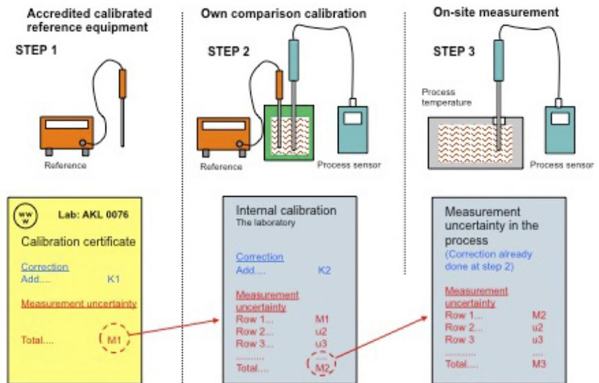
However, remember that the measurement uncertainty increases quickly with every comparison. The images above illustrate how measurement uncertainty is added to the chain at each step you take away from the accredited reference calibration.
