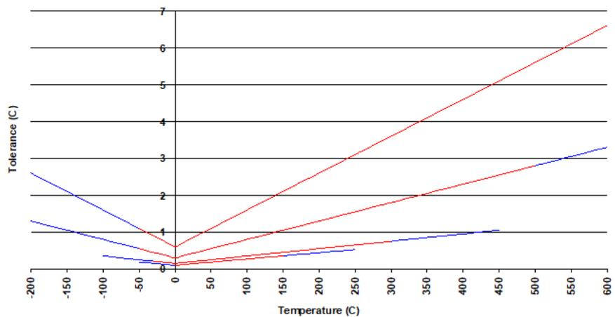
The tolerances of Pt100s according to IEC 60751 (2008) shown in graphic form. As a comparison, the positive tolerance limits according to Class 1 for types K and N thermocouples have been added as a dashed line. However, the platinum resistance thermometer is much more stable than the corresponding thermocouple.
