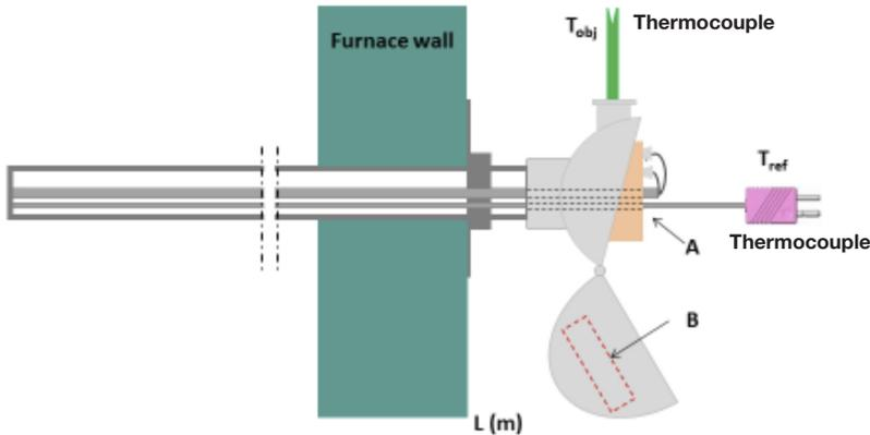
The reference sensor is inserted inside the extra tube that is inside the existing terminal block, see A.
