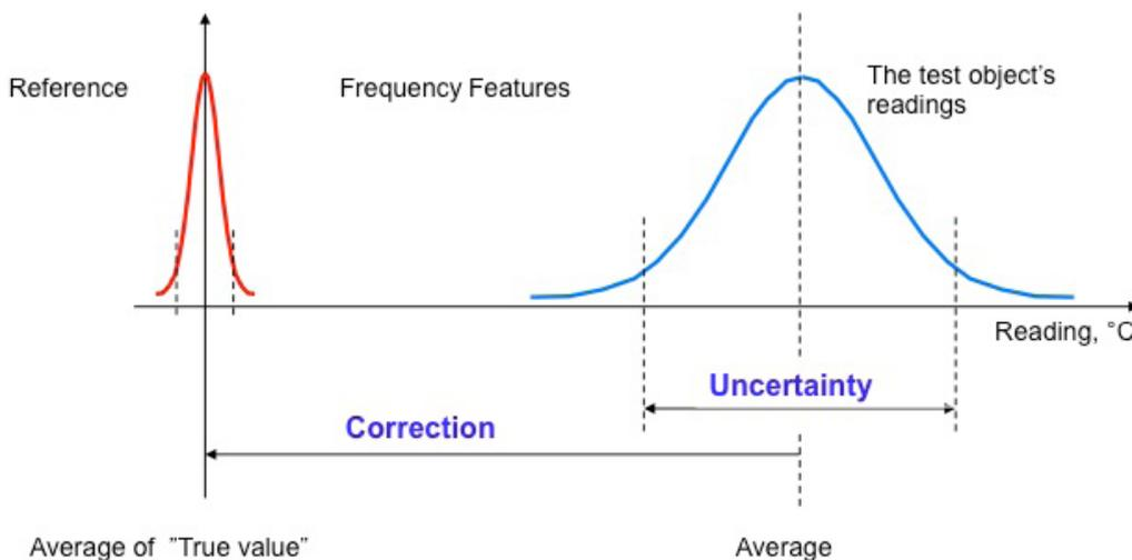
The figure shows the concepts of correction and measurement uncertainty in a comparative calibration. You obtain the spread around the mean values by repeating the readings a large number of times. The spread is caused by the chance measurement errors that are introduced with every reading.
