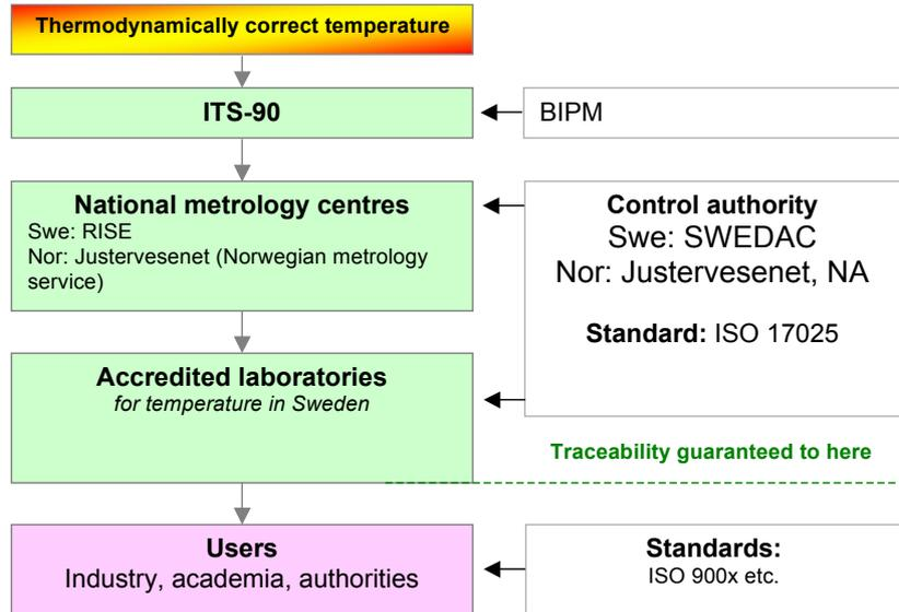
This figure shows how temperature is made traceable to ITS-90 via various calibration bodies. The link to the thermodynamic temperature is via BIPM's research project.
