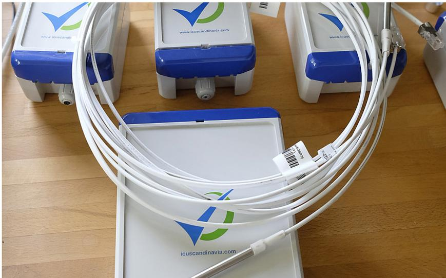
*The sensor, a special version made by Pentronic, supplies digital signals to nodes in the wireless temperature measurement system Boomerang.*
