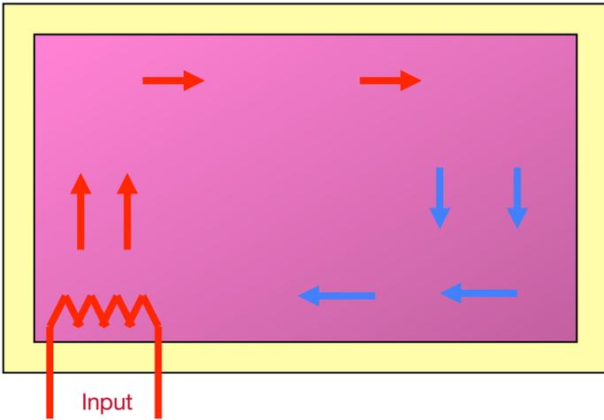
This figure shows an example of convection in an electrically heated hot water storage tank. The heat exchanger or immersion heater heats the water, whose molecules become more spread out due to their increased vibrational energy. Their density is thereby decreased and the hot fluid rises. When the fluid cools due to heat loss or heat extraction to a heat exchanger, the molecules become packed more tightly due to their reduced vibrational energy and they sink.
