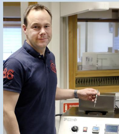
Lars Grönlund with the new calibration bath, which improves measurement accuracy when calibrating temperature sensors with short insertion depths.
