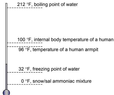
*Fahrenheit's mercury-in-glass thermometer with the reference points that were apparently used.*
