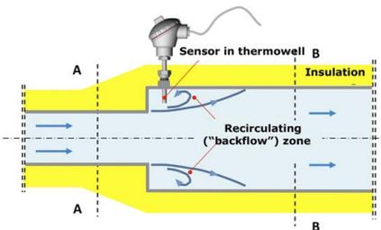
careful when installing thermowells and other components that disrupt the flow. One example is discussed in [Ref 2].
