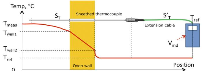
Figure 2. A general diagram of where in a thermocouple circuit the temperature signal is created. The most accurate measurement is achieved if the temperature gradients are located only along the length of the calibrated thermocouple.
