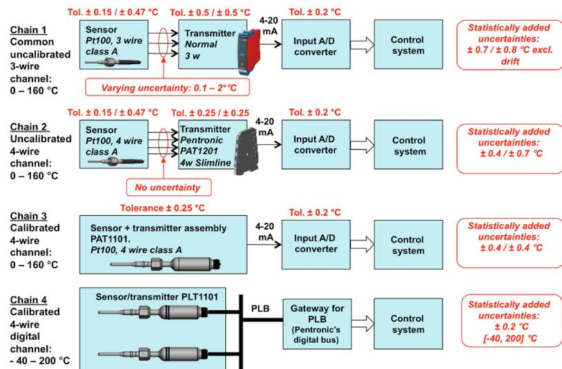
Figure 1. The figures show how we can sharpen the measurement chain from a measurement uncertainty  $\geq 0.81^\circ\text{C}$  down to  $\pm 0.2^\circ\text{C}$ . By using additional calibration points, Measurement Chain 4 can be pushed down to  $\pm 0.05^\circ\text{C}$ . In all cases there will be additional uncertainties due to the probe tip's design and installation.
