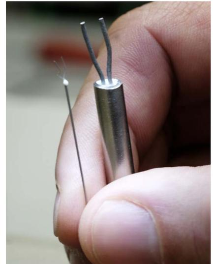
*The thin sheath material is 0.5 mm in diameter. The wires are scarcely visible to the naked eye and are welded under a microscope.*
