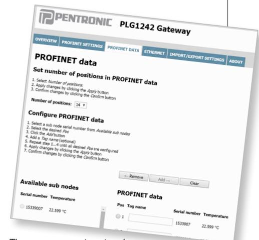
The measurement system is configured via a Web interface.
