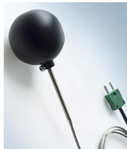
An example of a globe thermometer (50 mm) here with a thermocouple inserted into the centre of the globe. The globe thermometer should be freely installed in the air.
