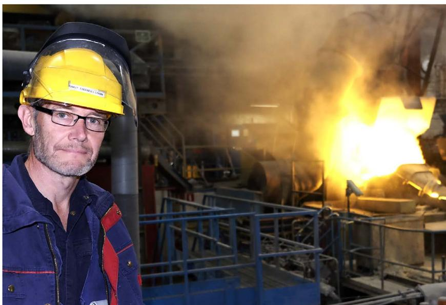
"We must be sure that the temperature stays within specific margins," says Ronnie Emanuelsson. Behind him the contents of one of the furnaces are being poured into a holding furnace for the casting of brass blanks.
