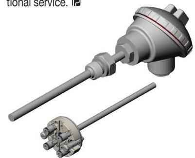
Figure 4. DIN 43772 (2000) describes various types of construction of sensors designed to operate in pipes and vessels. Shown here is a modified "form 2" (previously "form B") with a short neck and replaceable Ø 6 mm measurement insert. The air gap between insert and protection tube is eliminated by a metal bushing to improve heat transfer to the Pt100 resistor.
