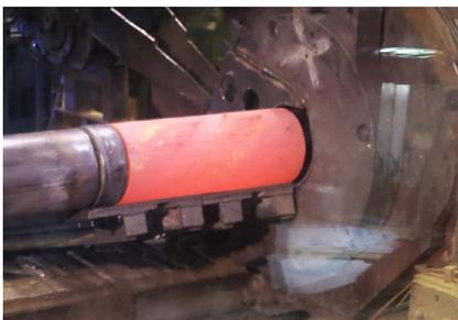
A heated brass blank before it is extruded to make profiles.
