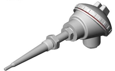
Figure 5. A thermowell's protruding section up to the probe tip has a resonance frequency, in this case two. The wake frequency of the flow influences the sensor with oscillations, which are governed by the construction, material and measurement environment. The ASME PTC 19.3 TW (2010) standard presents a method for determining if the wake frequency is limited enough not to initiate destructive resonance effects.
