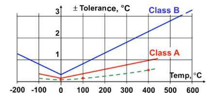
Figure 3. The diagram shows a typical behaviour of a platinum sensor in IEC Class A (the green dashed line). Three calibration points are shown (marked in red) within the interval 0–400 °C. Platinum is so stable that the points are sufficient to define the measurement properties within the whole range. See heading Calibration above discussing measurement uncertainty in the points.
