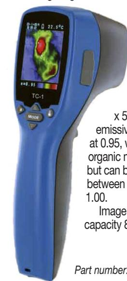
the temperature distribution is shown on the display, which is 40 x 50 mm. The emissivity is preset at 0.95, which covers organic materials but can be adjusted between 0.10 and 1.00. Image storage capacity 8 Gb.
