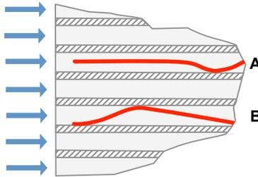
Figure 1. Catalytic converter channels with thin sheathed thermocouples (red) inserted from the rear against the flow direction.
