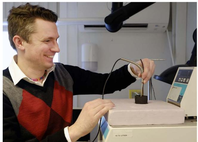
David Graaf maintains traceability of the temperature readings by calibrating in a water bath against an externally calibrated reference sensor.
