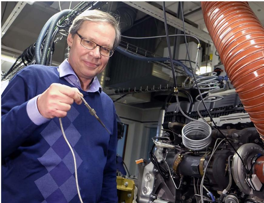
Temperature sensors are becoming more and more critical to engine development. They must measure correctly, react quickly and tolerate sudden increases in engine revs. Volvo's Mikael Svensson holds an exhaust gas sensor developed by Pentronic.
