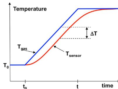
Figure 1. The gas temperature and sensor temperature when the gas temperature is changed in the form of a ramp.
