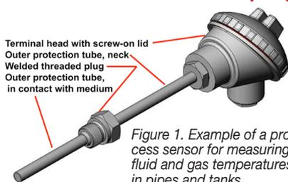
Figure 1. Example of a process sensor for measuring fluid and gas temperatures in pipes and tanks.
