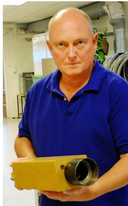
Per Johansson shows the camera that has made Gedvelop the world leader in the measurement of mass flow rates in the manufacture of fiberglass insulation.
