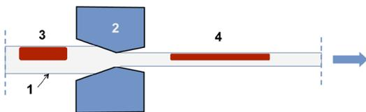
Figure 1. To suit the diameter to commercially used measurements, a thermocouple wire or a metal-sheathed thermocouple (1) is drawn through draw plates (2) equipped with smaller and smaller holes. An unavoidable impurity (3) from the alloy melt will also therefore in principle be reduced radially according to the draw plate hole. This thereby increases the length of both the impurity and the wire. See (4).
