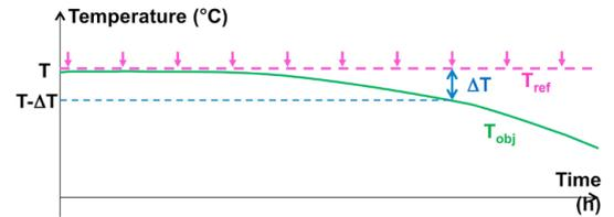
Figure 2. The pink dotted line is the reference temperature  $T$ . The solid green line shows the calibration object’s degeneration over time. If we take brief measurements (say 15 minutes) at regular intervals with the reference thermocouple, its operating time will be very short and its properties will be stable. We can then monitor the degeneration and decide at what  $\Delta T$  the calibration object must be replaced.
