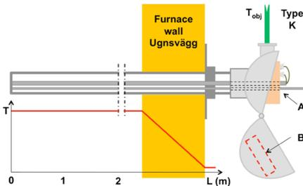
Figure 1. Thermoelectric voltage is almost always only created inside the furnace wall where the temperature gradient slopes ( $\neq 0$ ). Both the measurement object  $T_{obj}$  and the reference thermocouple  $T_{ref}$  take measurements under conditions that are as identical as possible. There are terminal blocks equipped with an extra hole for inserting the reference thermocouple into position, see A. When using a transmitter the solution can be to mount it inside the lid, see B.
