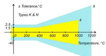
Figure 1. A graph showing the tolerances in accordance with IEC 60584 for types K and N thermocouples in class 1 (yellow) and class 2 (blue). Note that class 1 is limited to 1000 °C. Above 1000 °C a thermocouple in accordance with class 1 does not need to conform to class 2
