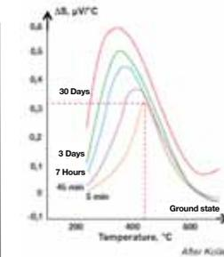
Figure 3. The SRO phenomenon's influence on type K thermocouples at various temperatures and exposure times. Already after five minutes at 450 °C sensitivity  $S$  has increased by 0.3  $\mu\text{V}/^\circ\text{C}$ .
