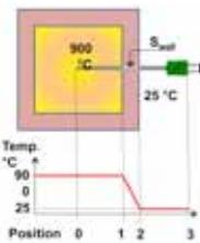
Figure 1. A thermocouple measures the temperature difference between its end points. In accordance with Equation (1) we get:  $E = S_{0-1} (900-900) + S_{1-2} (900-25) + S_{2-3} (25-25)$  which gives  $E = 875 S_{1-2} = 875 S_{\text{wall}}$ . The signal is thus generated where the thermocouple passes through the wall.
