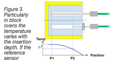
Figure 3. Particularity in block ovens the temperature varies with the insertion depth. If the reference sensor senses the bottom temperature (P1) and the measurement object is short (P2) due to a mounting component, they measure different temperatures even if both sensors otherwise have the identical construction. In this situation you can use the reference sensor to also measure at the P2 insertion depth and thereby minimise  $\Delta T$ .
